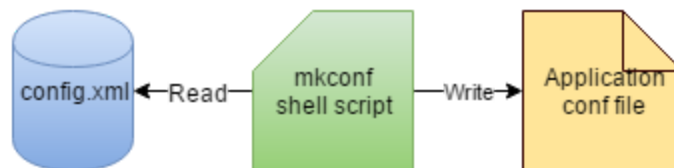
Figure 3. The shell script reads the data in config.xml and writes it to the application conf file.
